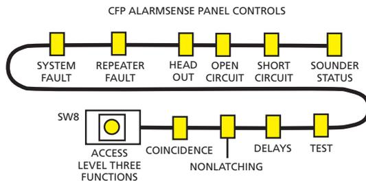
2. Continue pressing the ACCESS LEVEL THREE FUNCTIONS button until HEAD OUT light pulses. Any existing Zone Fault lights are suppressed and the zone light(s) for any zone(s) with a head out fault are illuminated, e.g. if a detector head has been removed on zone 2, Zone 2's Fault light will be lit.
