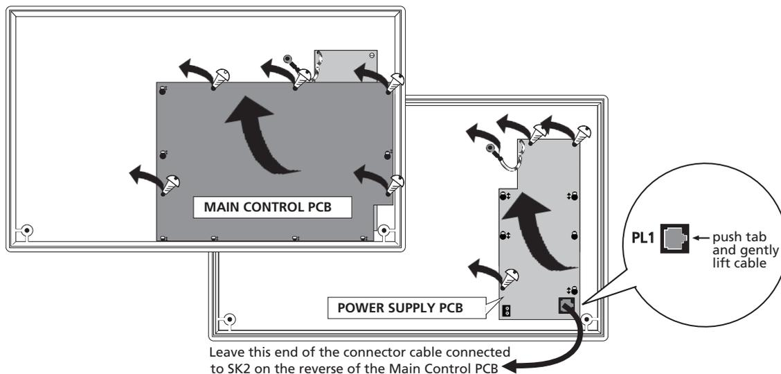
1. Take the fire alarm panel out of its box and undo the two lid screws using the Torx key provided. Remove the lid to expose the Main Control PCB (the Power supply PCB is located underneath).
