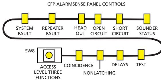
2. Continue pressing the ACCESS LEVEL THREE FUNCTIONS button until the SYSTEM FAULT light pulses.
