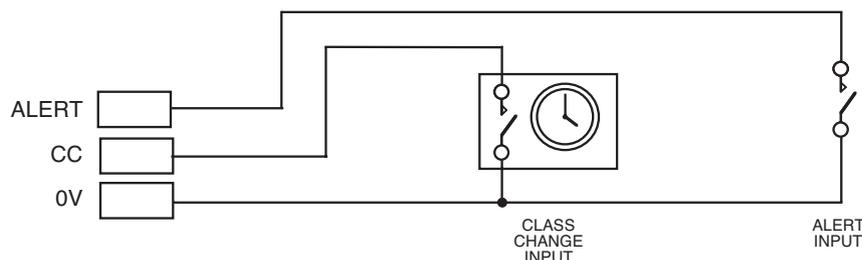
Connect the wiring for each input to the relevant 5mm connector block on the Main Control PCB and terminate their screens at the panel's base earth post (see page 13 for more details).
