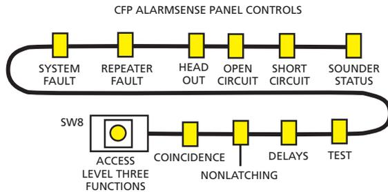
2. Continue pressing the ACCESS LEVEL THREE FUNCTIONS button until the REPEATER FAULT light pulses.
