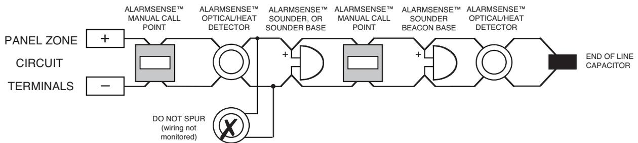
Connect an end-of-line (EOL) capacitor (provided in the panel 's accessory pack) across the terminals of the last device on each circuit to allow the wiring to be monitored. Unused zone circuits must also have an EOL capacitor fitted at the panel terminals.
