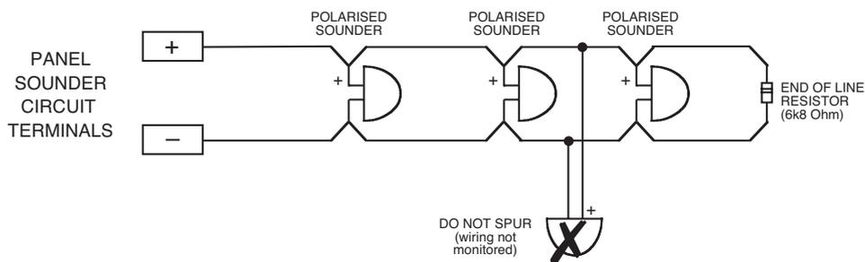
All sounders must be polarised as unpolarised sounders will show a sounder fault. Connect a 6k8 end-of-line (EOL) resistor (provided in the panel's accessory pack) at the end of each sounder circuit to allow the wiring to be monitored. Unused sounder circuits must also have an EOL resistor fitted at the panel terminals.
